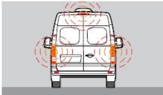
Emergency Stop Signal (ESS)
